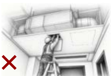
Conventional small modular trapdoors provide inadequate access
